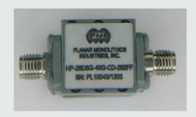
PMI Model HP-26D5G-40G-CD-292FF is a suspended substrate, high pass filter that has a passband of 26.5 to 40.0GHz. This model offers less than 2dB insertion loss while offering over 54dB of rejection at 20GHz and below. This model is supplied in an ultra-small housing that measures only 0.65" x 0.65" x 0.50" in size and is supplied with 2.92mm female connectors.
